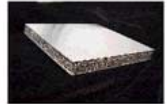
Al-face sheets joined to Gr-Foam with S-Bond™.
